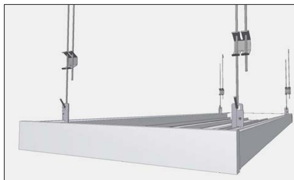
Figure 10. Atrium suspended on adjustable drop rods.
